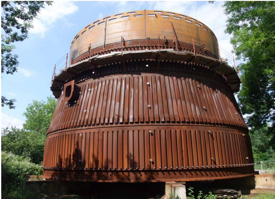
Figure 3. Preassembled shell of the hearth with the shell of the tuyère level thereupon.
