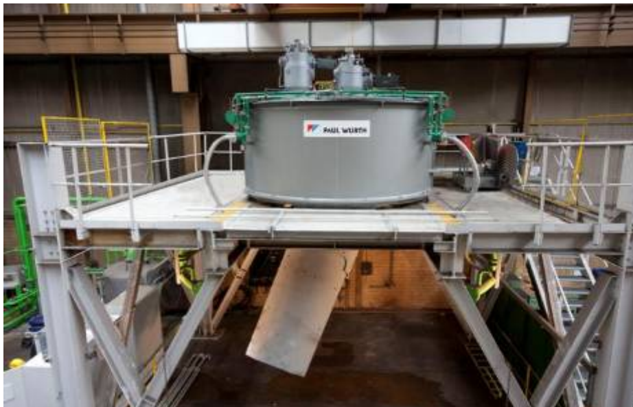
Figure 6. Paul Wurth BLT ® GEN3 gearbox and rotating chute at the test rig.
