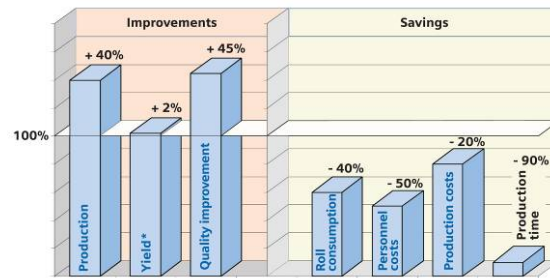
Figure 3: Savings and improvements after converting an existing pickling and tandem mill to a PLTCM.
