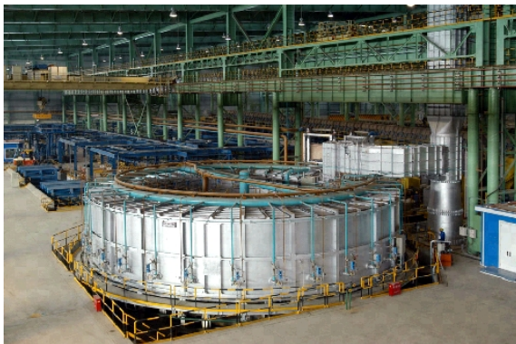
Fig 14. Rotary furnace overview and operating cycle for 316L, 5.0 mm.
