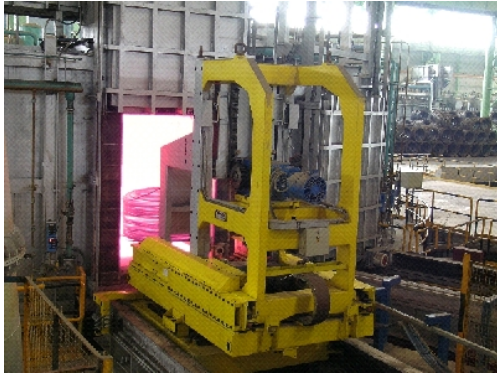
Fig. 8. Rotary furnace robot for coil charging
