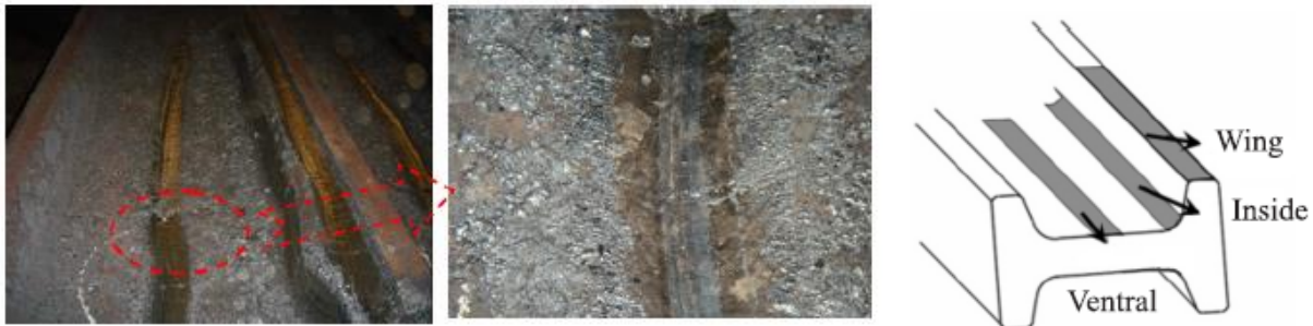
Figure 18. Scarfing for blowhole detection at Dragon Steel Corporation.
