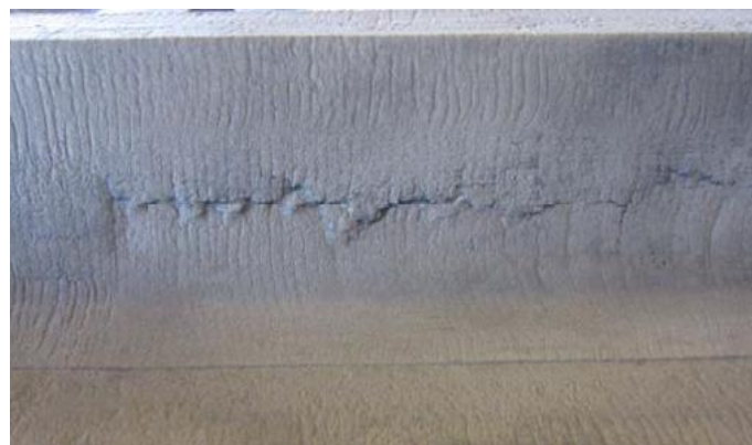
Figure 6. 670 mm wide beam blank with bleeding in the inner surface of the wing [11].
