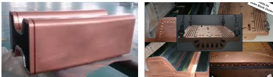
Figure 2. Molds for beam blanks. Left: Tubular mold. Right: Four plates mold.
