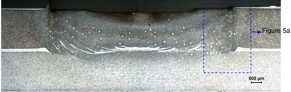
Figure 4. Cross section of the connection “S1” processed at: 2900 rpm, plunge depth 2.2 mm (0.2 mm), plunge rate 1.57 mm/s, time 2.8 s. Etching: Kroll solution.
