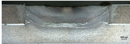
(d) Connection "S3" processed at 1900 rpm, plunge depth 2.2 s, plunge rate 1.57 mm/s, time 2.8 s.
