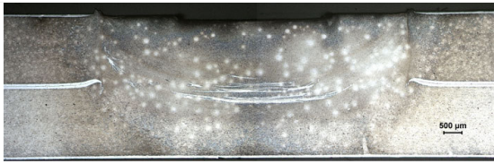
(b) Connection "S15" processed at: 1900 rpm, plunge depth 2.5 mm, plunge rate 1.04 mm/s, time 4.8s.
