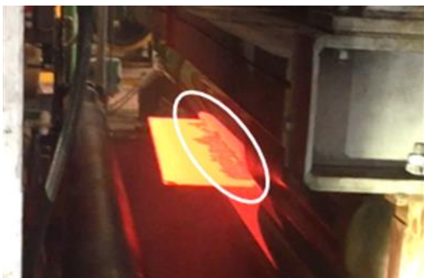
Figure 5. Seeping phenomenon of cooling water through the pinch roll
