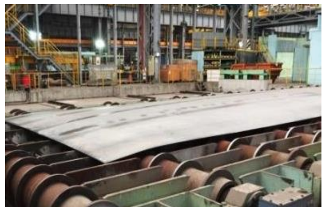
Figure 7. Flatness results after mid quenching test
