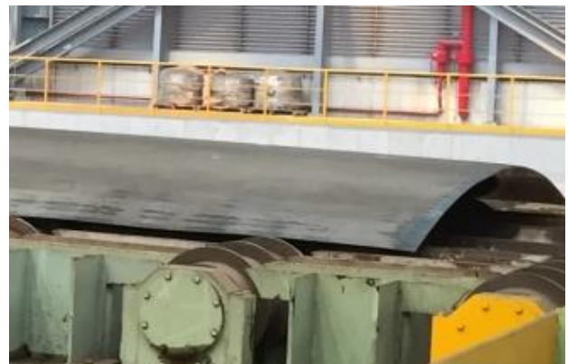
Figure 6. Flatness results after initial quenching test
