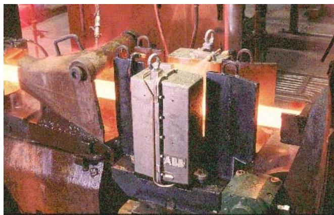
Figure 11. U Gauge in operation
