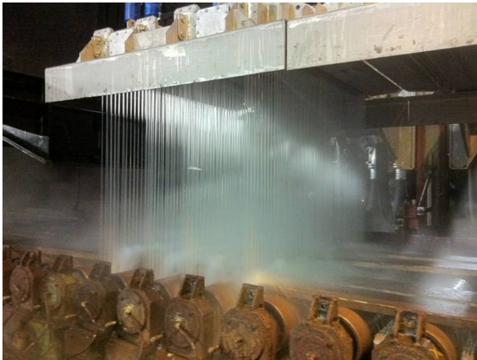
Figure 9. Test of fast cooling unit during start-up.
