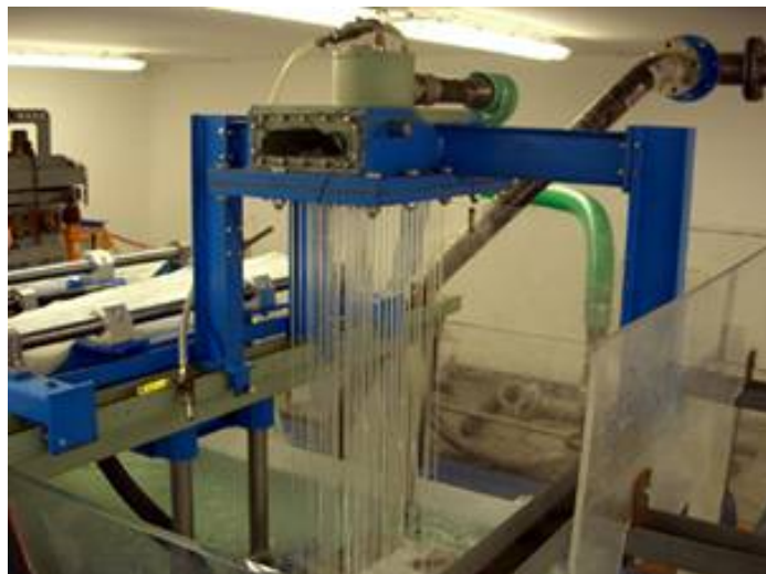
Figure 4. Trial at the continuous casting simulator at vatron, Linz.
