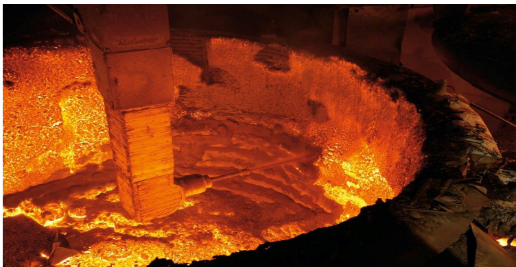
Figure 1 - EAF gunning operation
