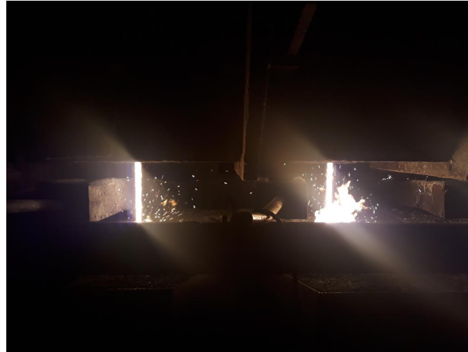
Fig. 6 Sparkling mold during casting. In left hand side strand liquid powder is used.
