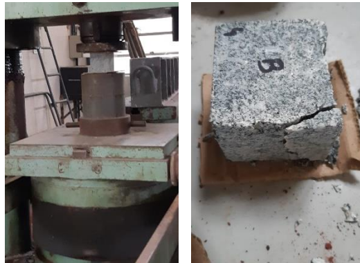
Figure 3. Uniaxial Compression Strength test
