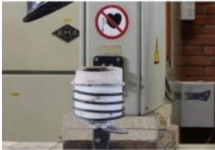
Figure 2. Induction furnace Hüttinger 10kW.
