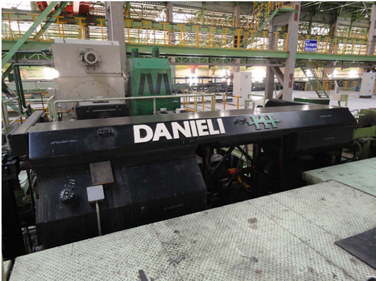
Figure 5. TMB Finishing Block.
