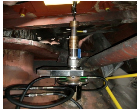
Fig.8 Top video camera at ArcelorMittal Dofasco
