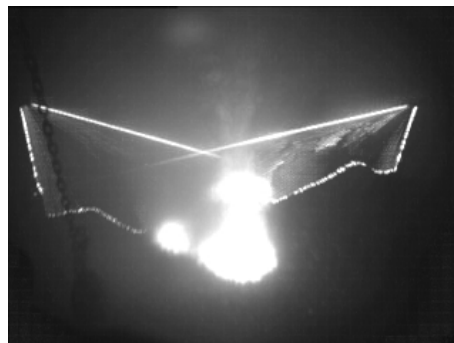
Fig.14 An burden slipping image in 2200m 3 BF at Baotou
