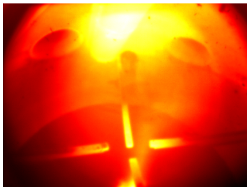
Fig.9 Thermal Camera Image of 5800m 3 BF in Shagang
