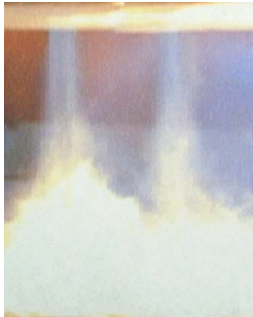
Figure 2. Oxyfuel flames in Direct Flame Impingement.
