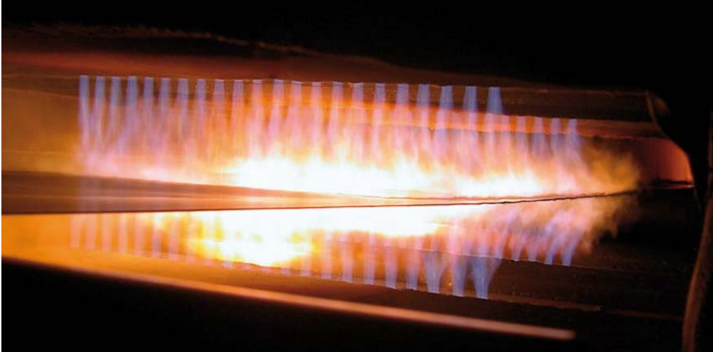
Figure 6. A look inside the DFI unit in Finntrop: Oxyfuel flames are heating directly onto the moving strip, increasing the temperature more than 200°C.
