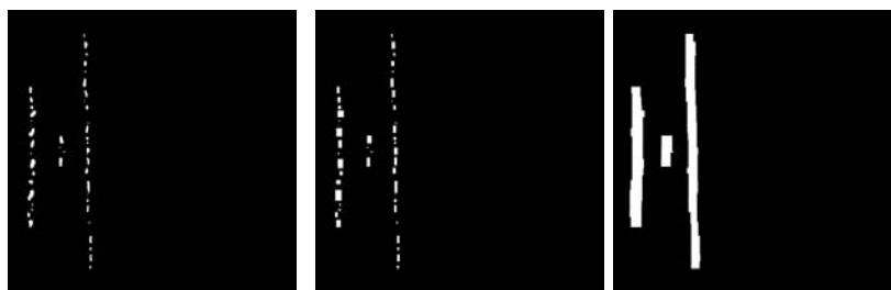
Figure 10 – Identification of stringers – Type B. a) 3 stringers. b) Each inclusion surrounded by its aligned convex hull. c) After horizontal dilation and vertical closing.
