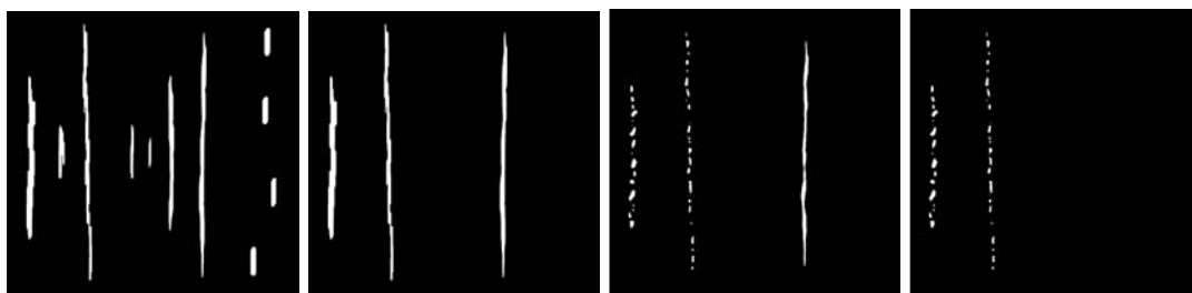
Figure 4 – Second processing step. a) After vertical dilation. b) Elimination of short objects. c) Intersection of the result in b with the original image. d) Type B S \geq 2.0 .
