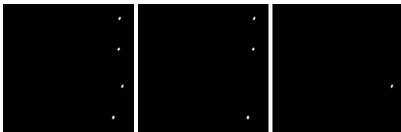
Figure 9 – Classification according to thickness. a) Type D inclusions. b) Thin series. c) Thick series.
