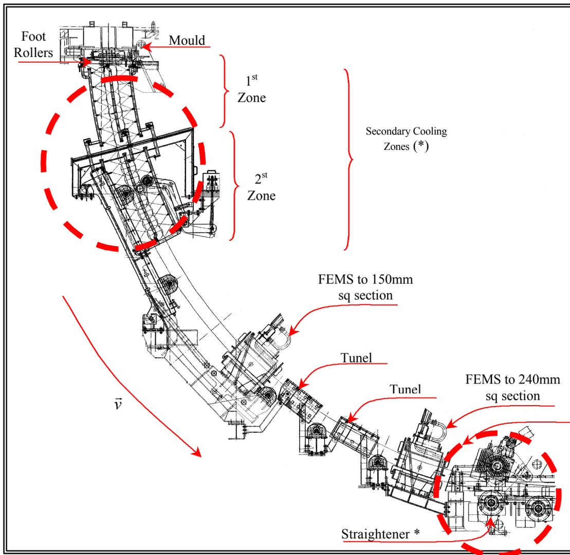
Fig. 3. Gerdau Aços Finos Piratini – CCM – Critical zones for surface cracks initiation/growth
