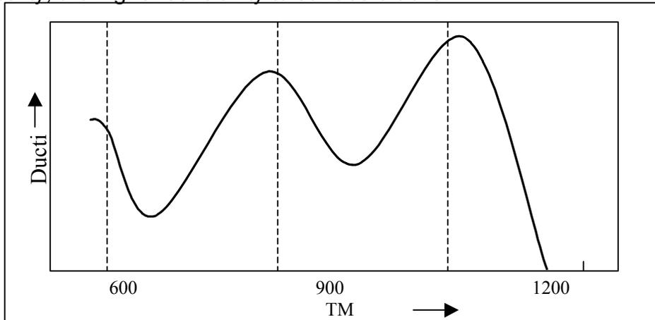
Fig. 4. Schematic representation of ductility troughs appearing in the hot tensile test in steels
