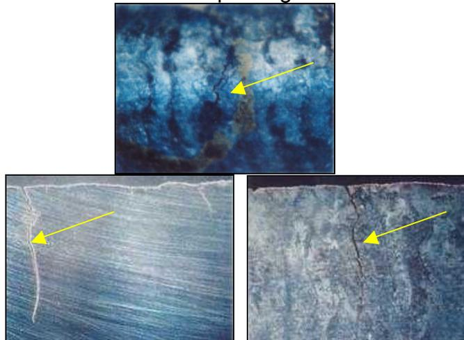
Fig. 2. Transverse Cracks at the bottom of oscillation marks, indicated by arrows, after acid pickling:
