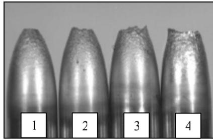
Fig. 8 – visual RA of the specimens after the tests
