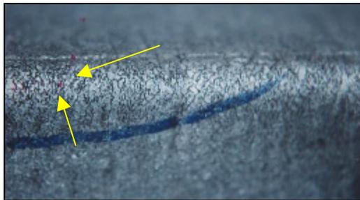
Fig.1. – Network cracks, indicated by arrows, presented at bloom surface after acid pickling
