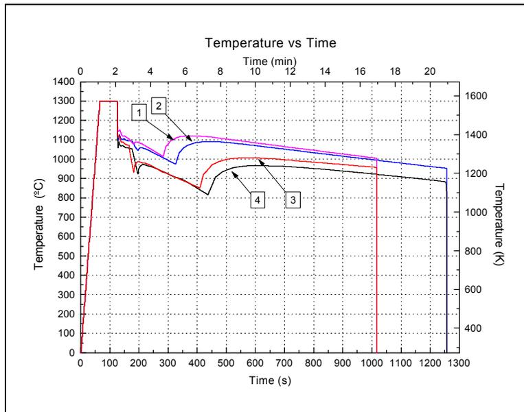
Fig. 7 – Thermal evolution of the casting simulation previous to tensile test
