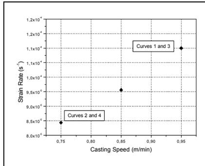
Fig. 6 – Casting Speed x Strain Rate applied in the CCM simulation test
