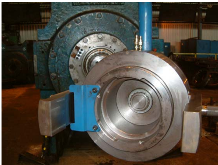
Fig 2 Hydraulic Tool arms that hook to the latches are shown on the outside.
