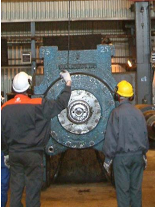
Fig 1 Traditional Method of Tightening Locknut
