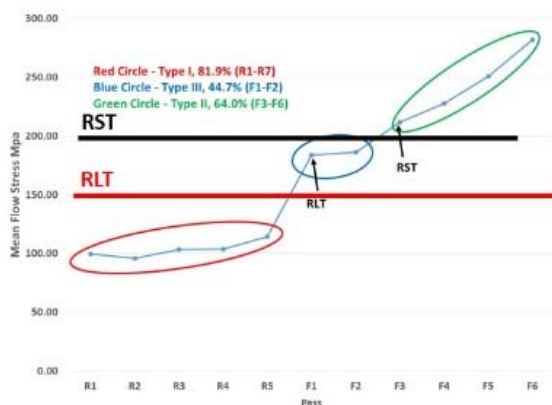
Actual 700 MPa YS 6mm hot strip coil MFS showing three recrystallization behaviors
