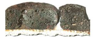
These test demonstrate that all the dunite charged as lumps and in the Sinter with the burden are molten as a flux in the belly and upper bosh of the blast furnace. Other more refractory fluxes stones do not have much chance to melt down and react before they reach the very high temperature zones in the lower bosh (above 1450°C). At this point it is too late to carry out effectively most of the functions for which fluxes are introduced.
