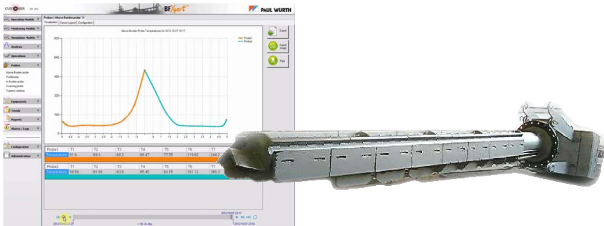
Figure 4. Above-burden Probe and graphical representation in BFXpert.
