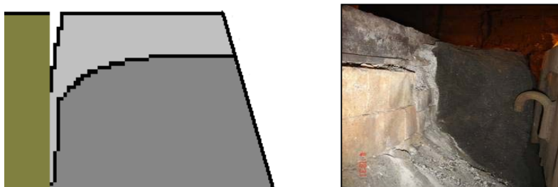
Figure 2. Oxidation process through working lining and safety lining interface
