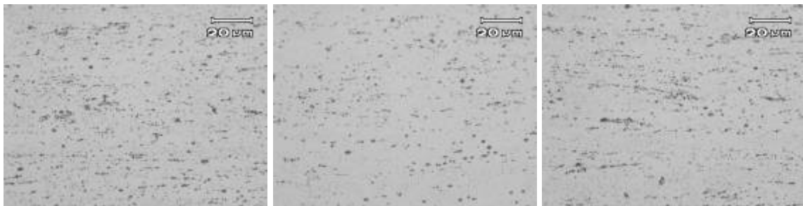
(a) (b) (c) Figura 12. Temperatura de Ho 520°C. (a) 10°C/h (b) 20°C/h e (c) 60°C/h.
