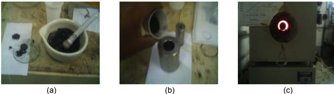
**Figure 1** – (a) Fines blending; (b) Indeflexible steel matrix; (c) Tubular electric furnace
