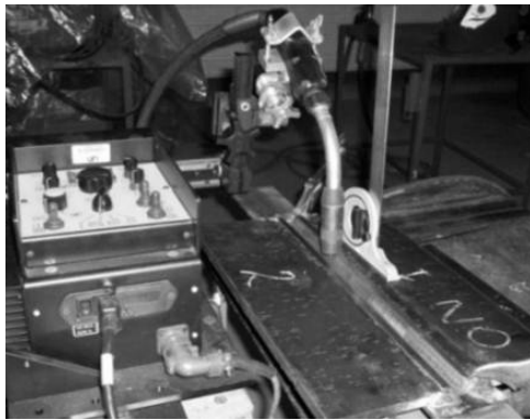
a) Experimental setup b) Bead-on-plate Figure 1. Experimental setup for joint and bead on plate testing.
