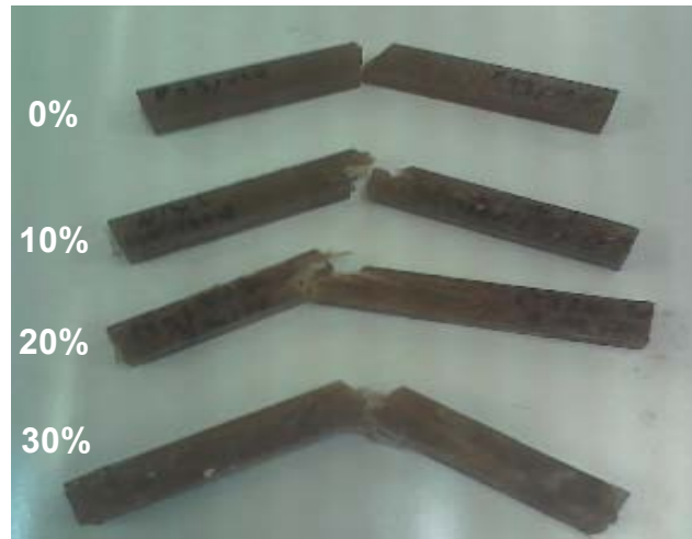
Figure 4. Microstructure aspect of strong alkali treated (10% NaOH – 1hour) curaua fiber reinforced polyester specimens after Charpy impact tests.
