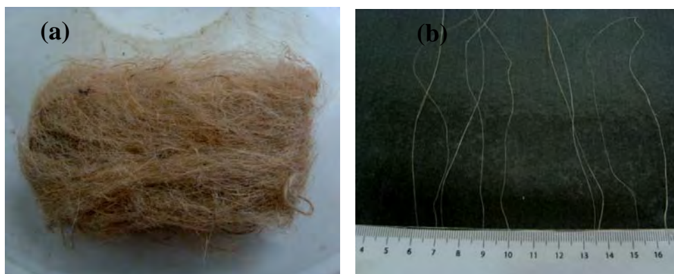
Figure 1. A bundle of as-received (a) and individually separated jute fibers (b)
