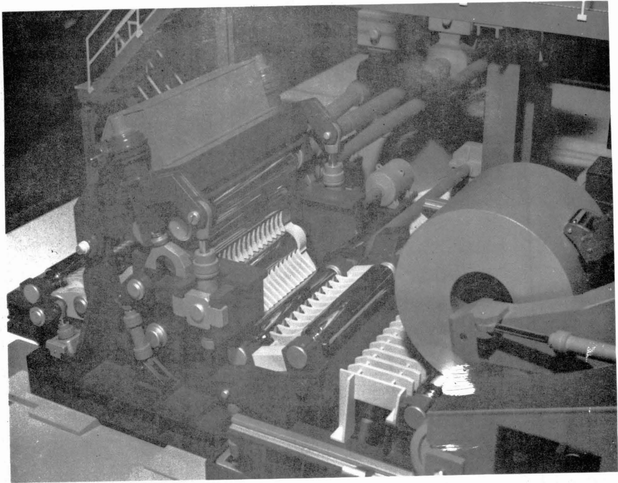
Fig. 5 Model of Coilbox bending roll arrangement
