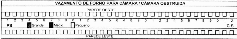
• Figure 3 Data sheet showing gas leakage from ovens to combustion flues
