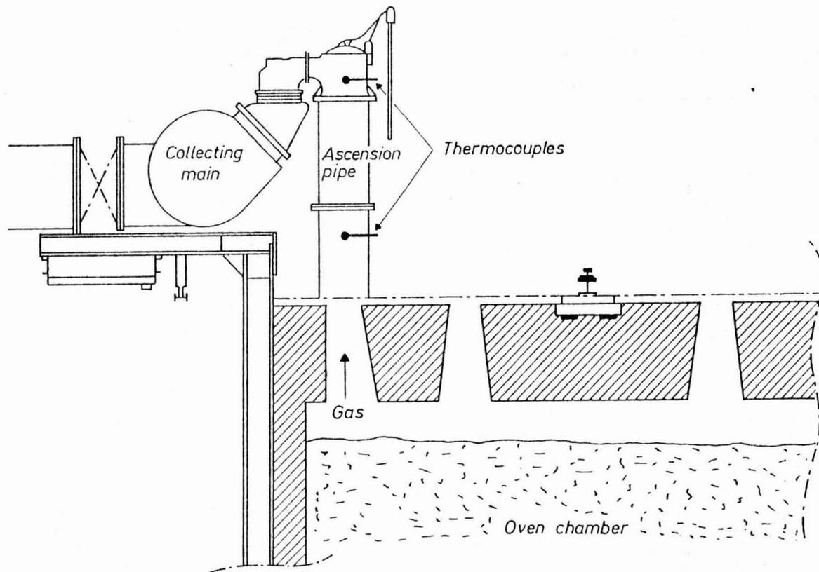
*Fig.8 Thermocouples' position in the ascension pipe*
