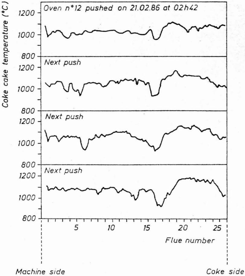
Fig.16 Temperature profiles observed during successive pushes of an oven
