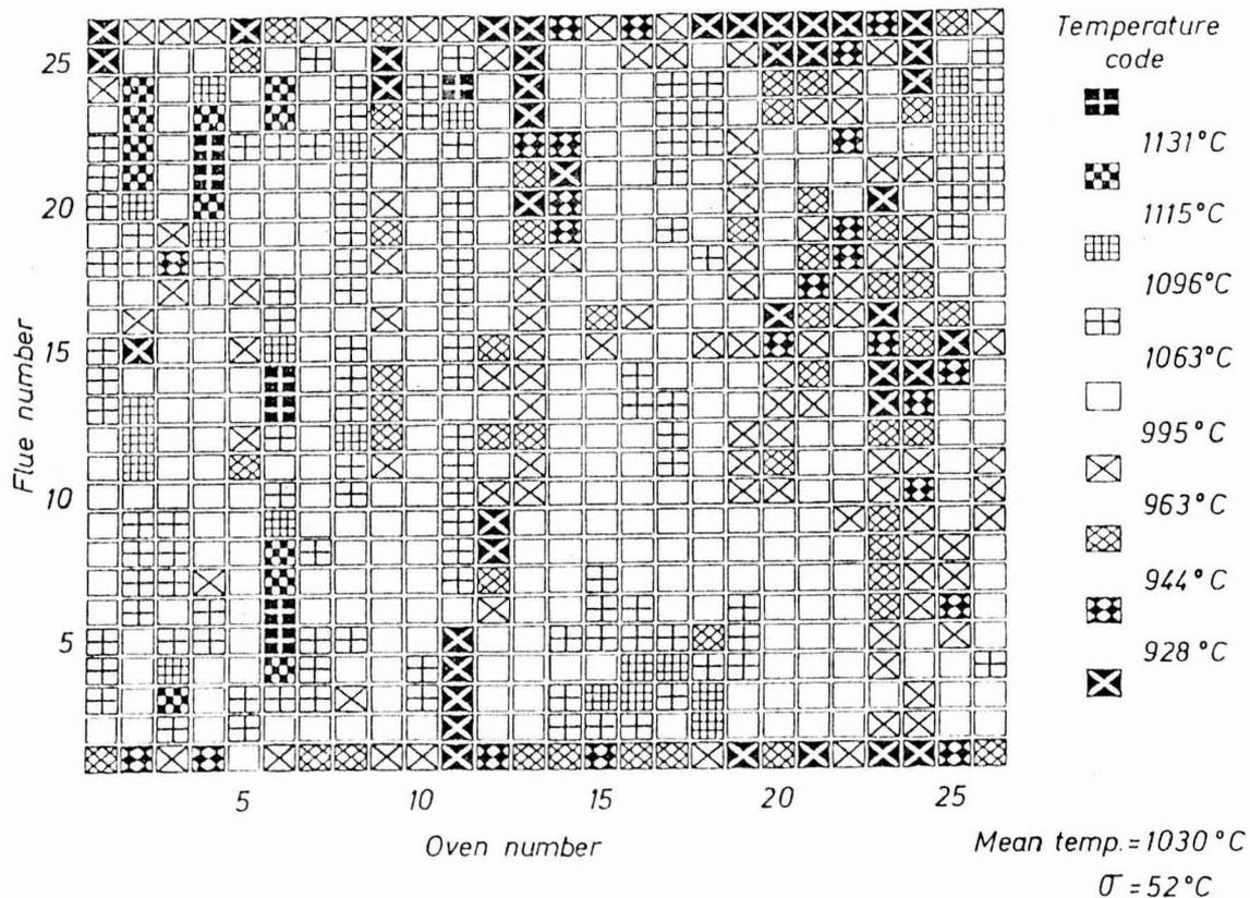
Fig.14 Temperature map of a coke oven battery
