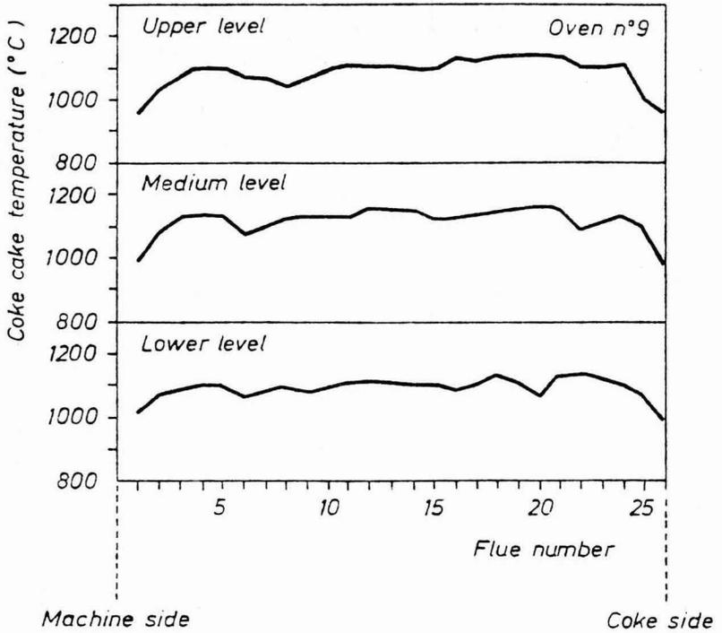
Fig.13 Typical coke cake temperature profiles
