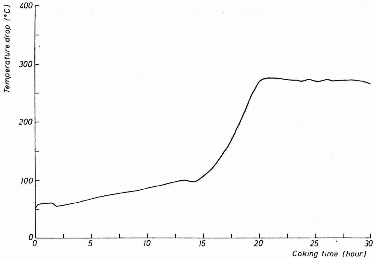
Fig.9 Gas temperature drop in the ascension pipe during carbonization process
