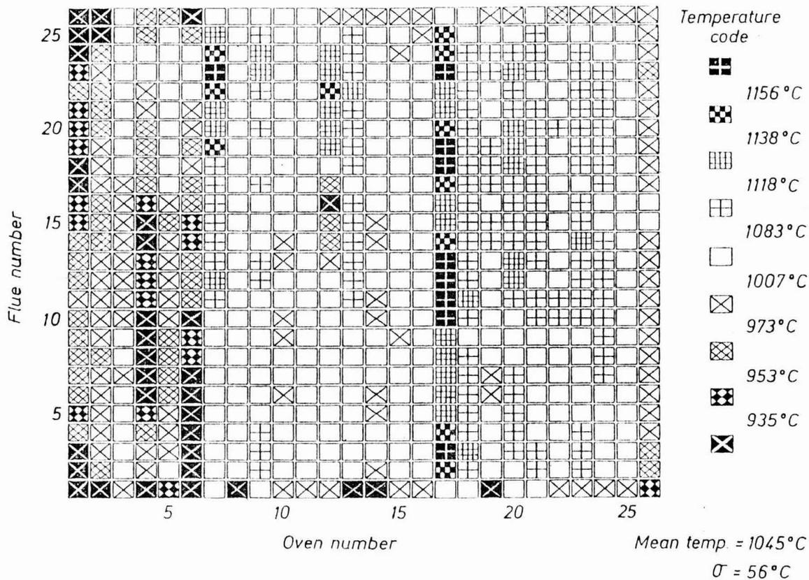
Fig.15 Mean temperature map of a coke oven battery for eight successive pushes
