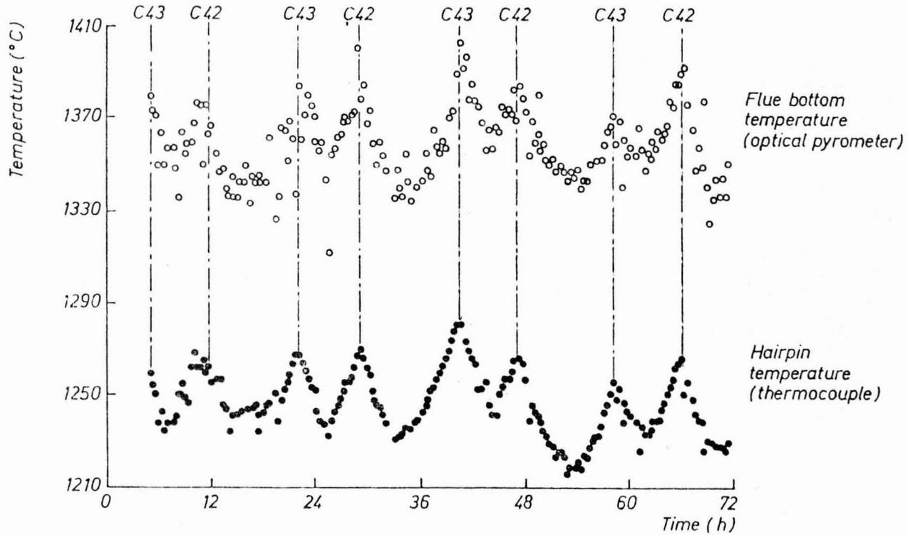
Fig.5 Flue temperature evolution
