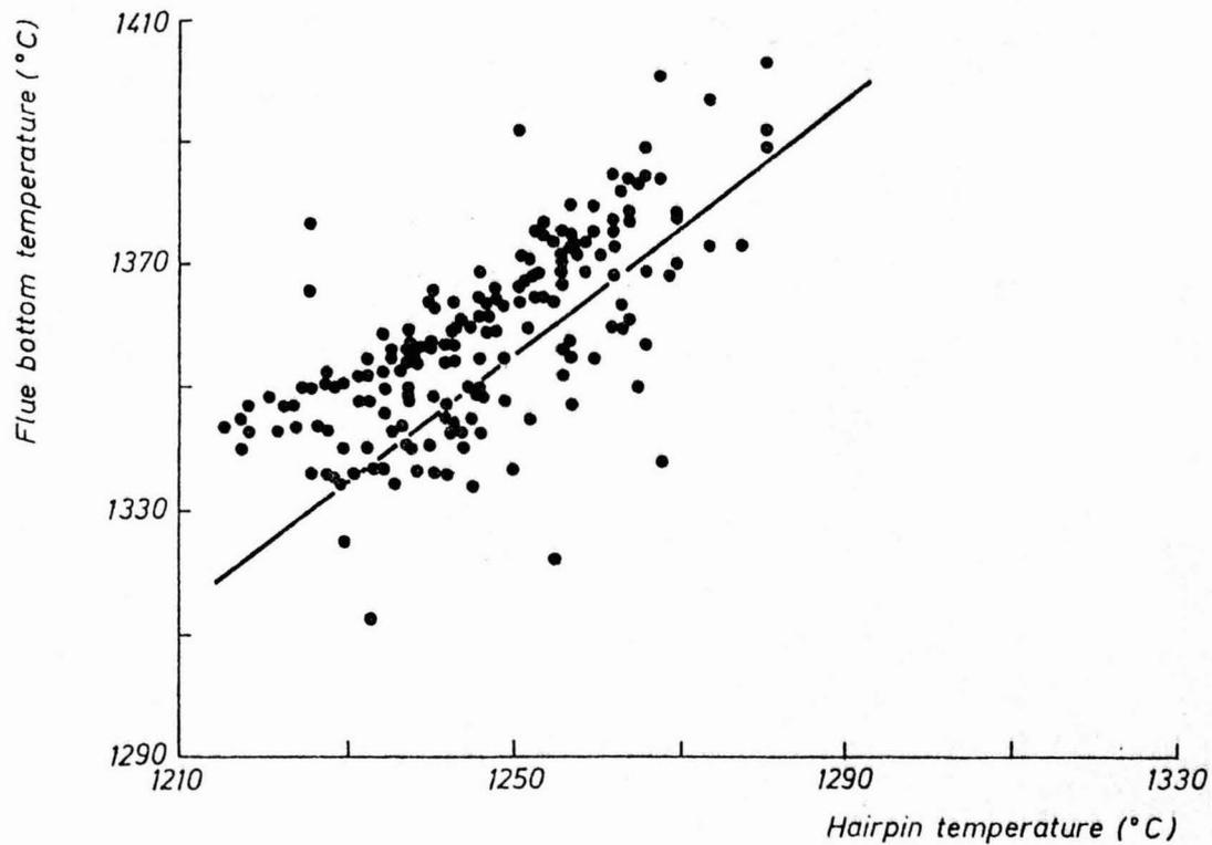
Fig.6 Correlation between hairpin and flue bottom temperatures
