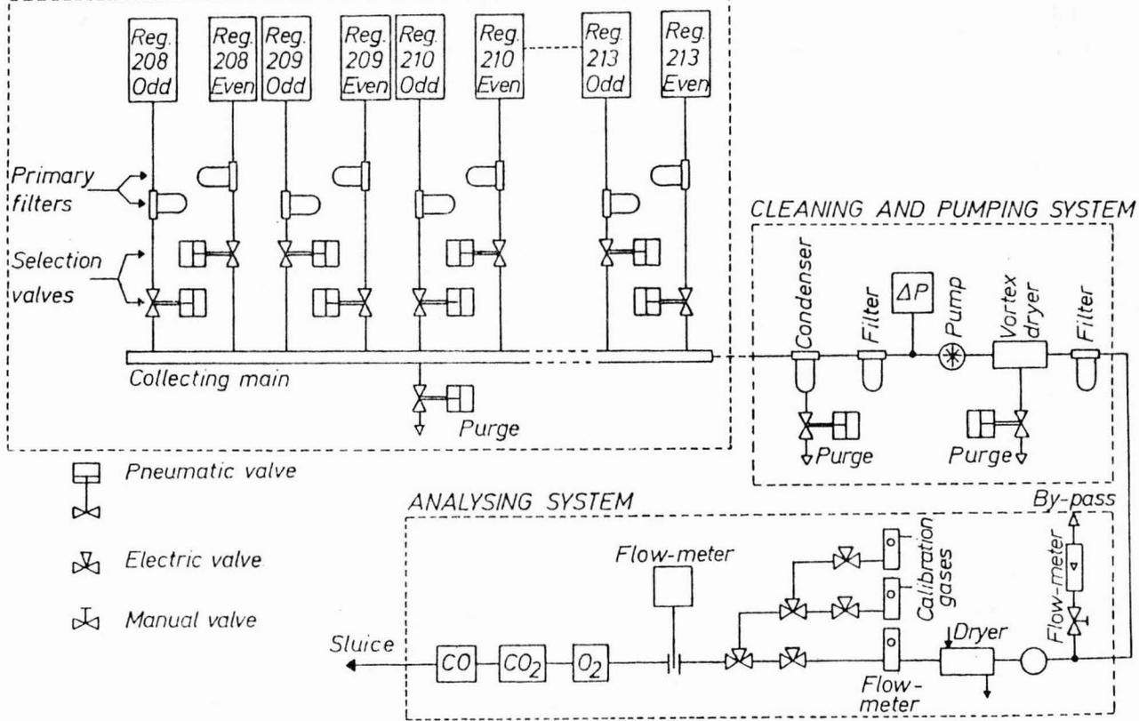
Fig. 11 Waste gas analysis at regenerators' outlet
