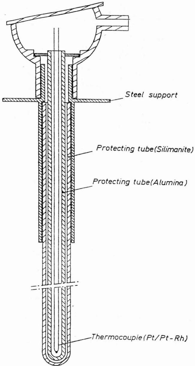
Fig.2 Temperature probe
