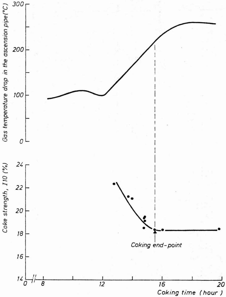
Fig.10 Coking end-point detection
