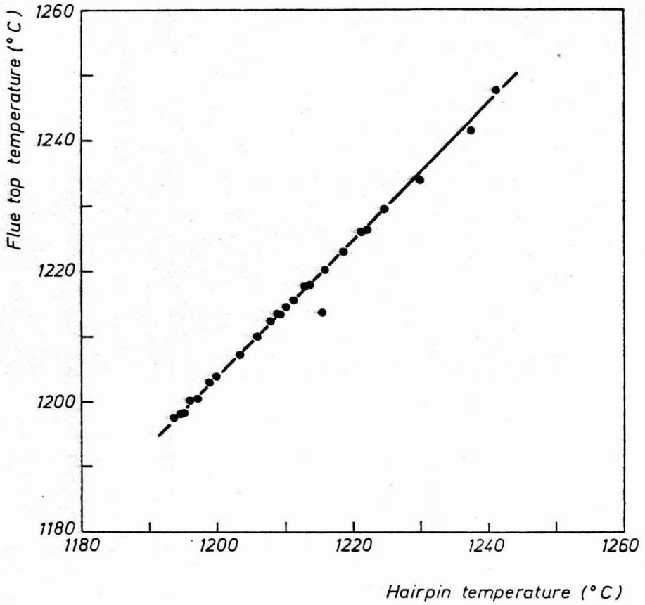
Fig.7 Correlation between hairpin and flue top temperatures
