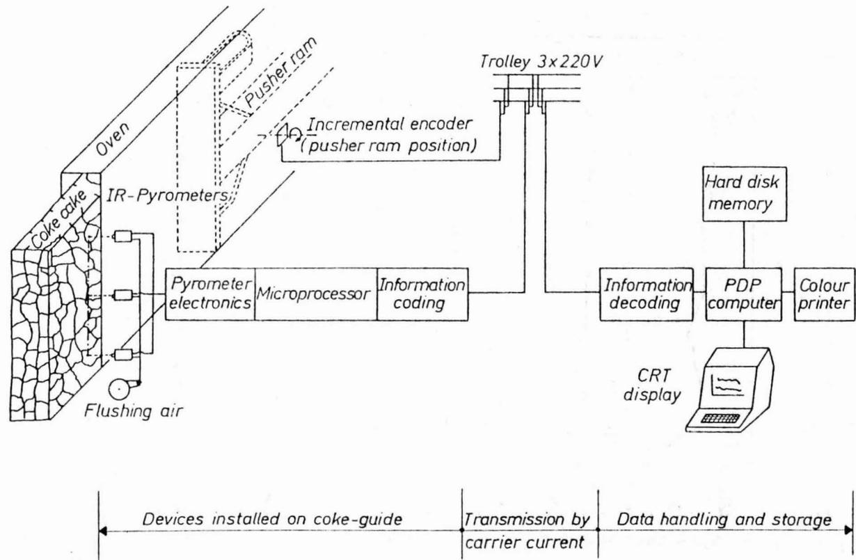
Fig.12 Schematic layout of the COTHERM system
