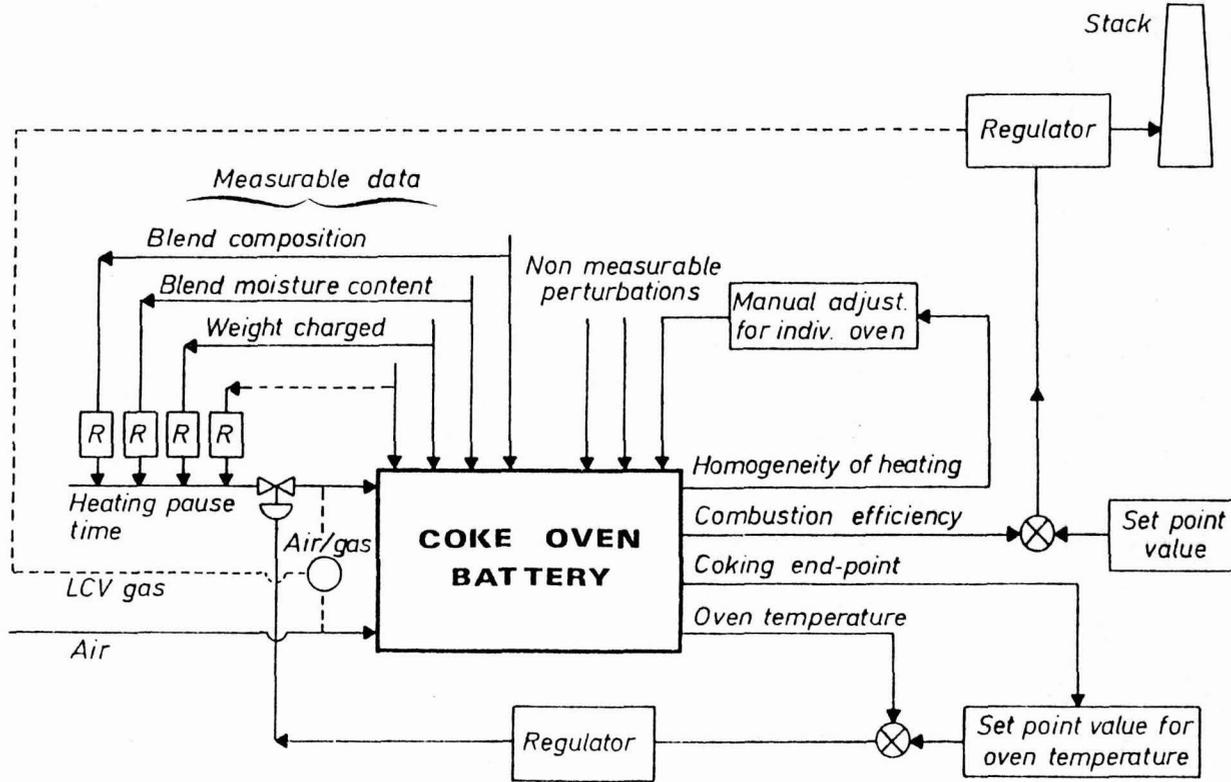
Fig.1 Schematic representation of CRM system for coke oven control
