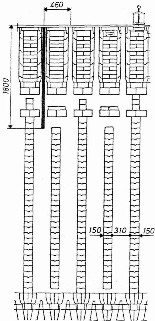
Fig.4 Thermocouple position at the top of the heating flue
