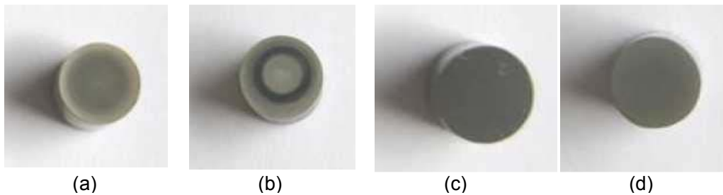
Figure 3. Typical characteristic after nitriding by DCPN for (a) AISI 1020 steel, (b) AISI 316 steel and by CCPN for AISI 1020 and AISI 316, (c) and (d).
