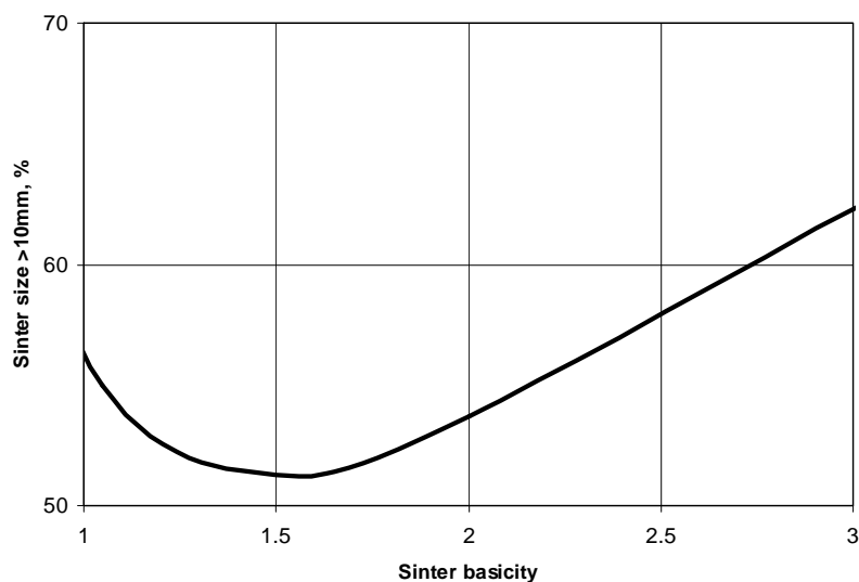
Figure 3. Relationship between sinter strength and sinter basicity. (1)
