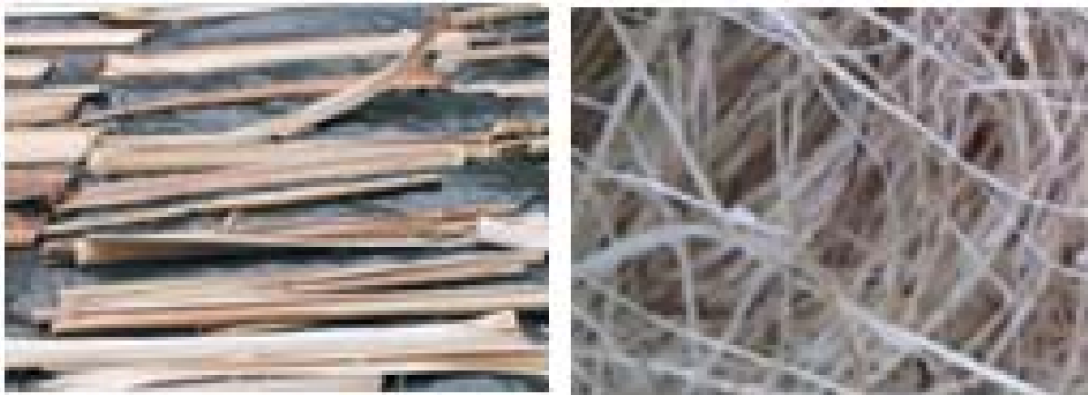
Figure 2. (a) Longitudinal stalks sectioned from the pseudostem; and (b) banana fibers separated from the stalks.
