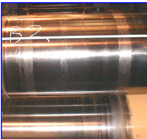
Figure 2: Work Roll Peeling
