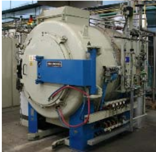
Figure 1. Horizontal furnace for nitriding using ZeroFlow process.
