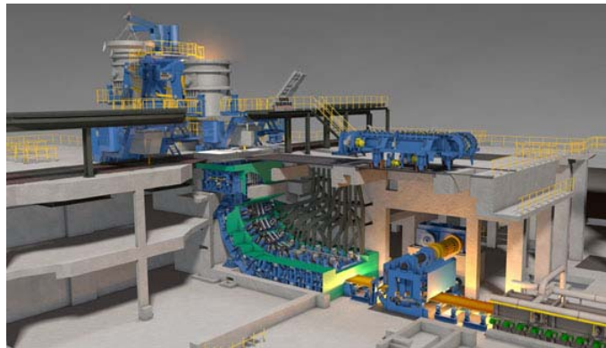
Figure 14: The CSP ® caster of VLB type combines the well-known thin slab technology with proven and new technologies
