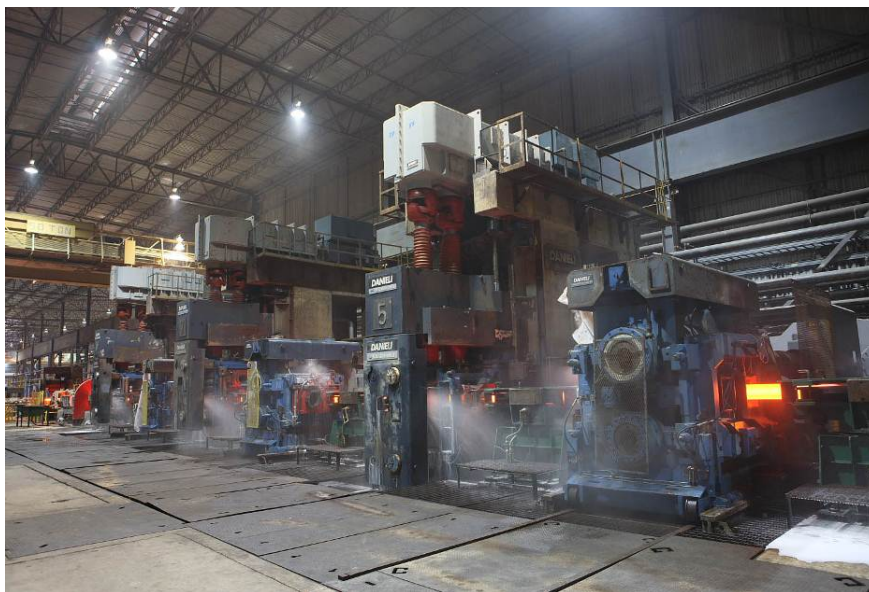
Fig. 6: Continuous finishing mill with SHS stands in H/V arrangement
