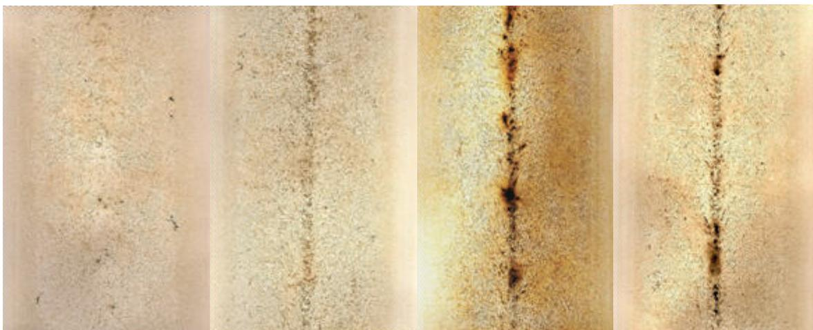
a) Main EMS @ 254 A    b) Main EMS @ 305 A    c) Main EMS @ 356 A + Brake    d) Main EMS @ 390 A + Brake
