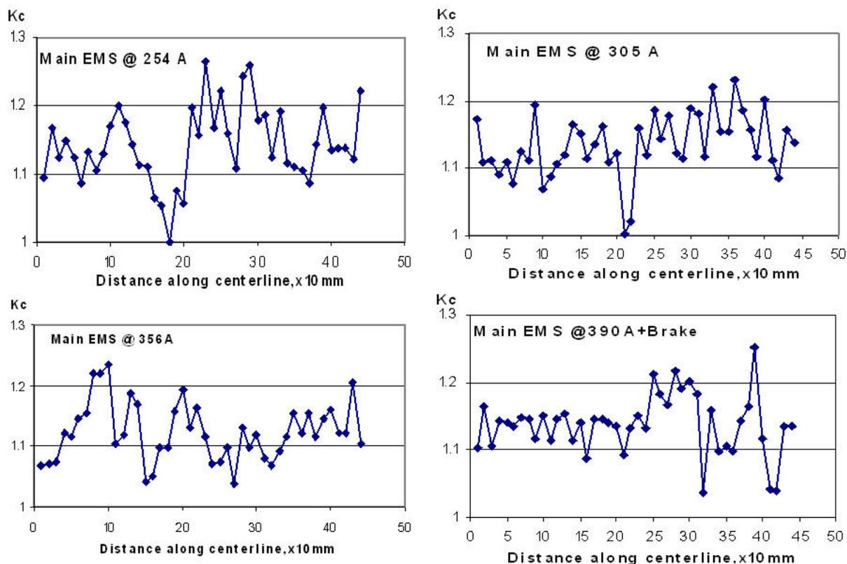
**Figure 5.** Centerline carbon segregation in the billets cast with different EMS settings
