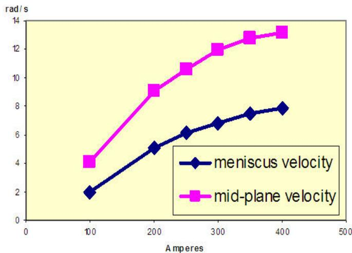
**Figure 3.** Stirring velocity in mercury vs. EMS current
