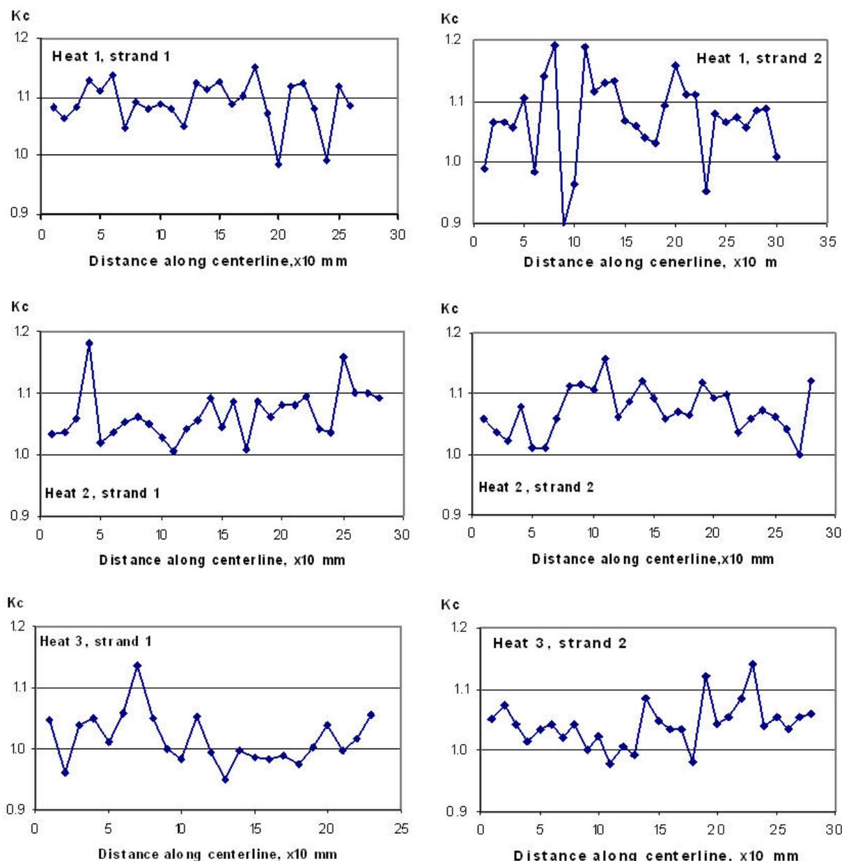
**Figure 6.** Centerline carbon segregation in the billet cast with the standard EMS setting of 390 A on the main EMS + brake
