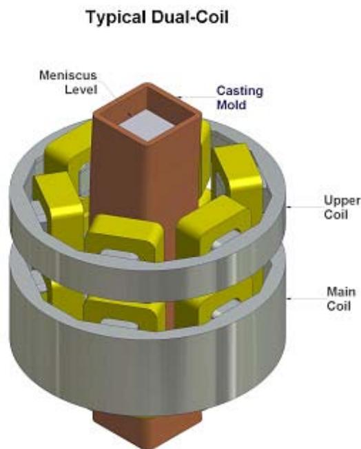
**Figure 1.** Schematic of dual-coil EMS
