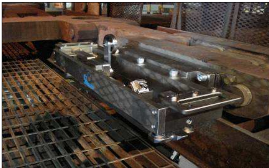
Figure 10 - Measuring assembly with 80 mm measuring range.
