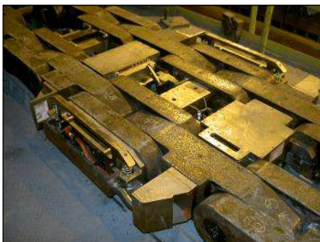
Figure 5 - New In-Chain system installed in dummy bar chain.
