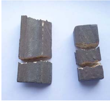
Figure 3 Results after thermal shocking for the coated sample
