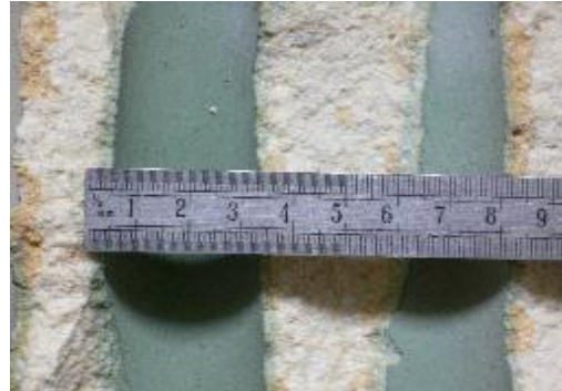
Figure 4. Structure of the coating infiltrated into the brick
