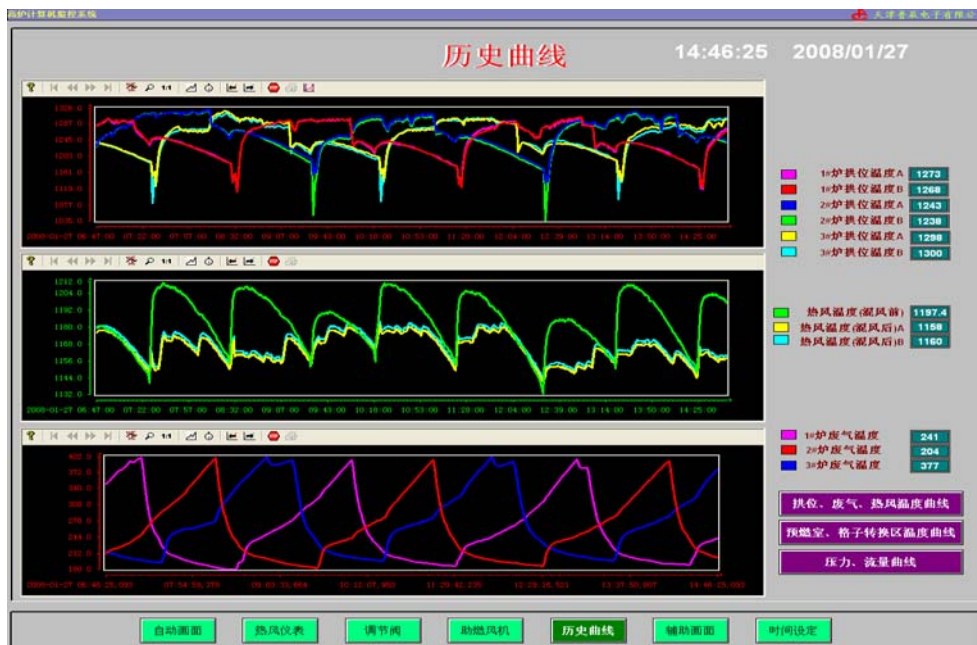
Figure 12 Some temperature distribution in hot stove with and without coating in a Chinese Steel Co.
