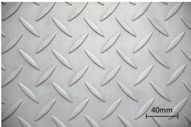
Figure 3. Photo of the roll-bonded clad checkered plate with a sandblasted and galvanochemically treated surface
