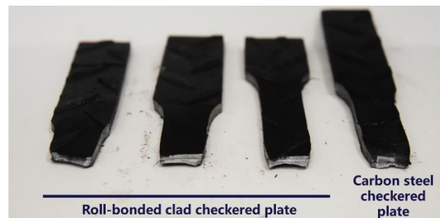
Figure 8. Fracture morphology of tensile test specimen
