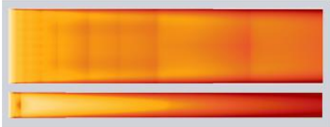
Figure 5: Calculated temperature profile of strand surface (top and side view, true colors)
