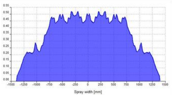
Figure 10: Spray pattern zone 3 - new nozzle types (120°)
