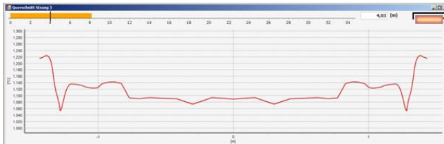
Figure 11: Surface temperature across strand width at 4m from meniscus using new nozzles
