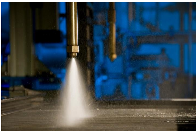
Figure 2: Measuring nozzles at the nozzle test stand
