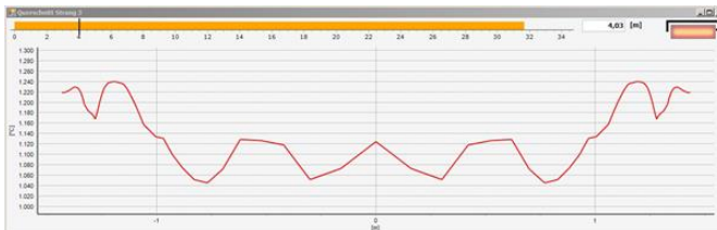
Figure 8: Surface temperature across strand width at 4m from meniscus using existing nozzles
