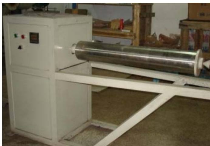
Figure 3. The drum to test the strength of coke after reaction.
