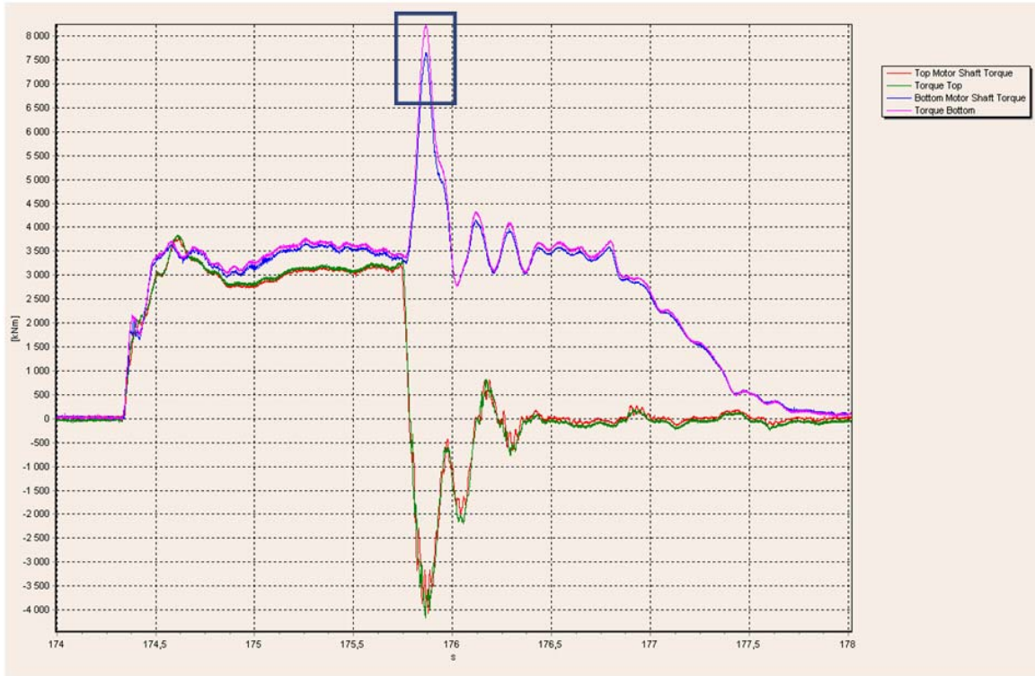
Figure 20. Torque measurement from a top motor cut event.
