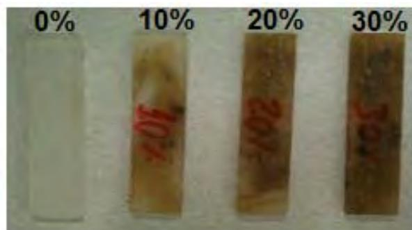
**Figure 2.** DMA specimens of epoxy matrix composites incorporated with different volume fraction of malva fiber.
