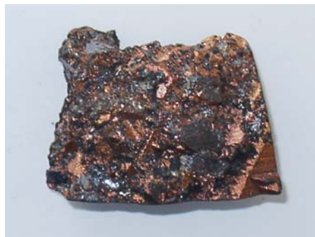
Figure 4. Pieces of TiN, TiC, Ti(CN) protection layer from BF.
