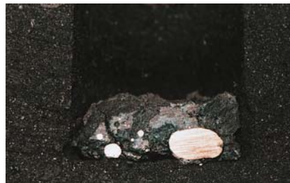
Figure 2. Lump ilmenite test. Crucible containing Slag, Fe and lump ilmenite.
