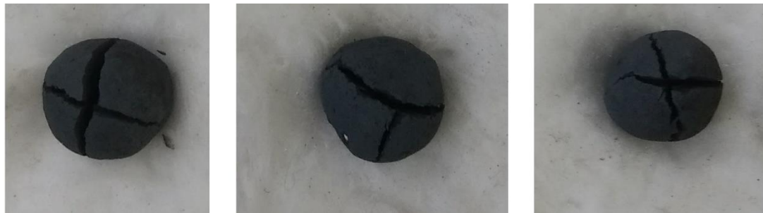
Figure 6. Some of the reduced pellets for basicity 1.5 and MgO 5%, showing major cracks.
