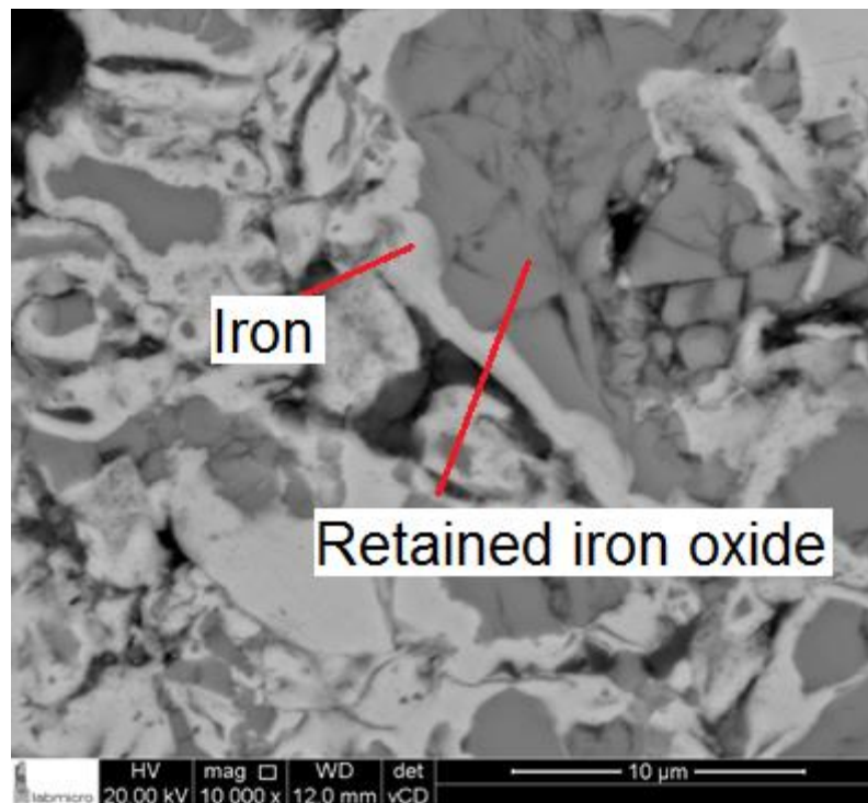
Figure 7. Crack within iron oxide matrix due to reduction stress.
