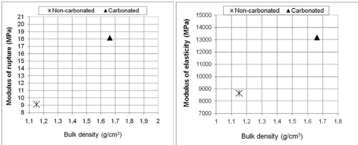
**Figure 1.** Average values modulus of rupture (MOR), modulus of elasticity (MOE) and and bulk density (BD) of the fibre–cement composites.
