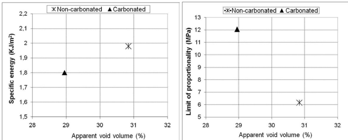
**Figure 2.** Average values of specific energy (SE), limit of proportionality (LOP) and apparent void volume (AVV) of the fibre–cement composites.
