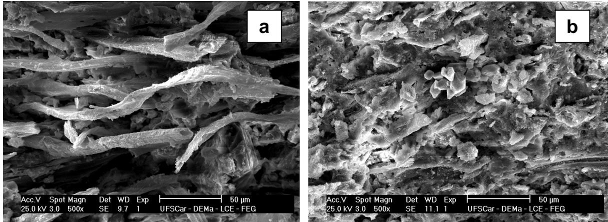
**Figura 3.** SE micrographs of the composite fracture surface (a) non-carbonated and (b) carbonated.
