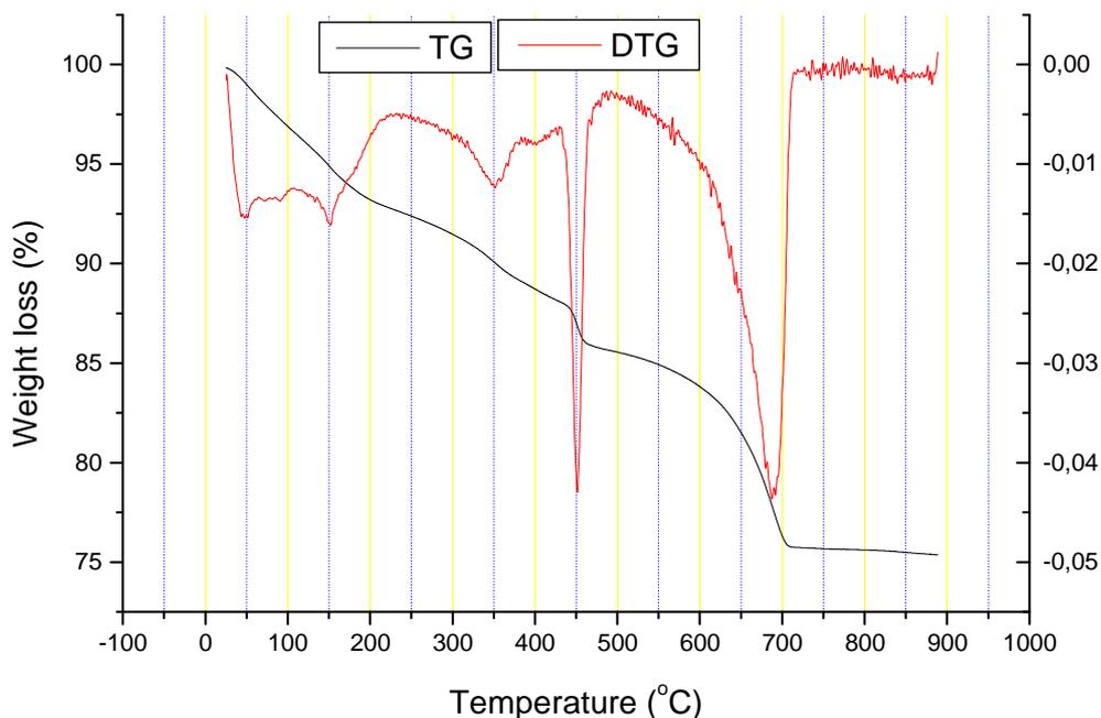
**Figura 5.** Weight loss of the non-carbonated composite.
