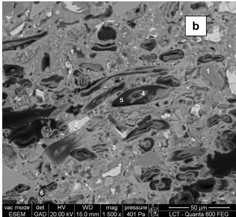
**Figura 4.** GAD micrographs of the polished cross-section of the composites (a) non-carbonated and (b) carbonated.
