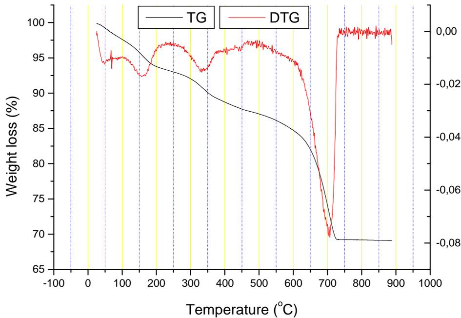
Figura 6. Weight loss of the carbonated composite.
