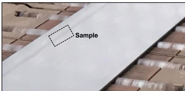
Figure 14: Plate with not uniform descaling.
