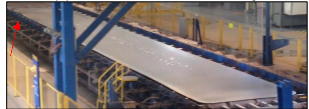
(c) Plate after hot leveler.
