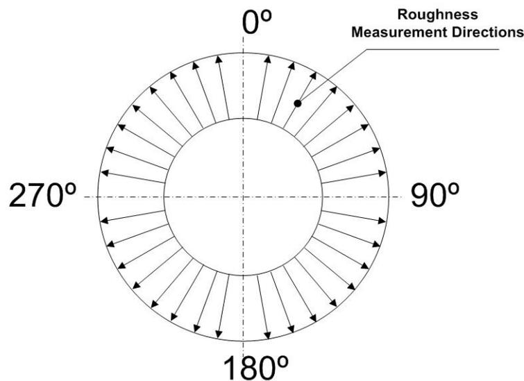
**Figure 1.** Directions used for the roughness measurements.
