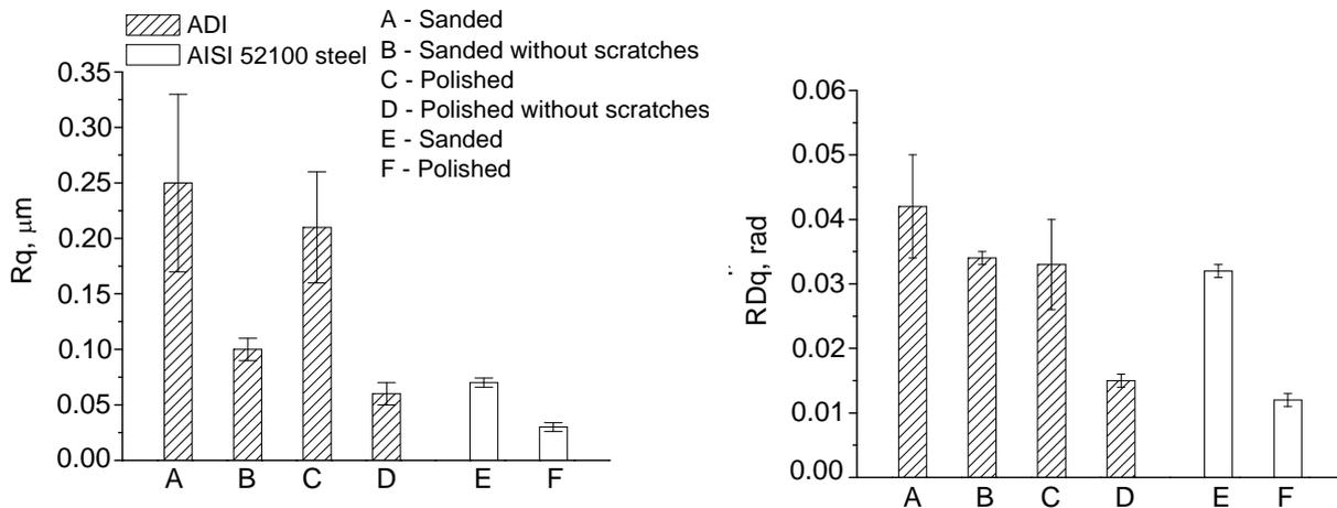
**Figure 5.** Effect of the scratches removal of the ADI profile regarding values of roughness parameters  $R_q$  and  $RD_q$ .
