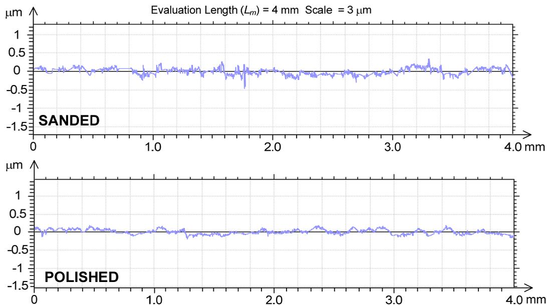
**Figure 4.** Profile of the ADI surfaces after the removal of scratches using the software.
