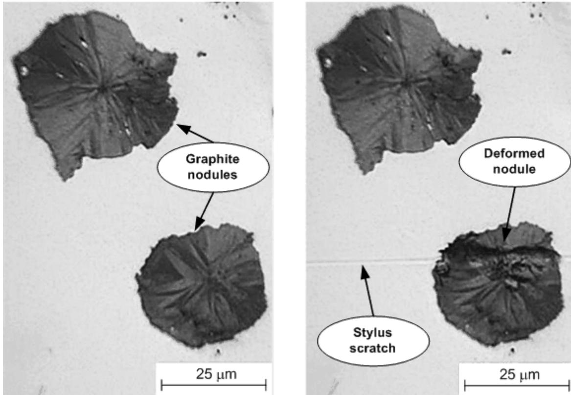
**Figure 2.** Image of deformed nodule of graphite during the roughness measurement.
